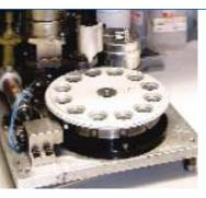
Lenses secured by highly precise automated adhesive dispensers
